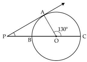
Ans: We know that the tangent at a point to a circle is perpendicular to the radius passing through the point of contact.
